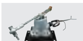
RUDDER ANGLE SENSOR
