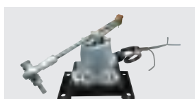
RUDDER ANGLE SENSOR
