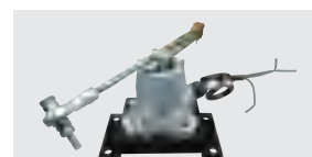
RUDDER ANGLE SENSOR
